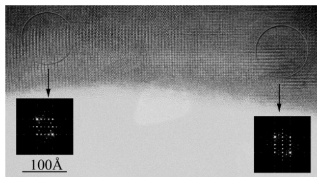
Figure 8. HREM micrograph recorded along the same zone axis as in Figure 7. FFTs calculated for different domains indicate microtwinning.
